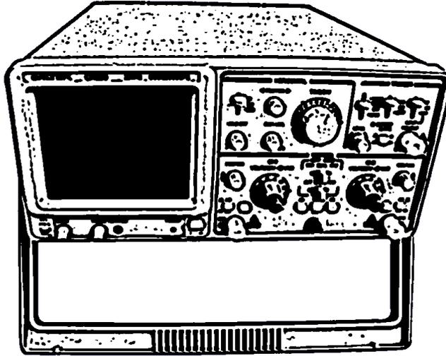
The device shown above is known as an *oscilloscope*, and the screen on the left shows a visual image of a signal or sound wave sent into its input. Eshaal is using it to view the sound waves generated by a microphone placed underneath a tank of fish.
